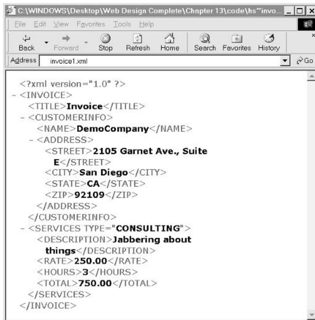
Figure 16-7. Well-formed XML example rendering
